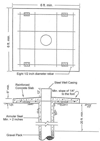
**Dimensions:** The slab must extend horizontally at least three feet from the center of the well casing in all directions.
