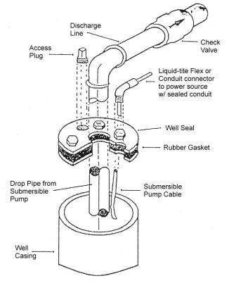
**Well Seal:** A properly sized well seal must be installed so as to provide a watertight seal between the casing and drop pipe.
